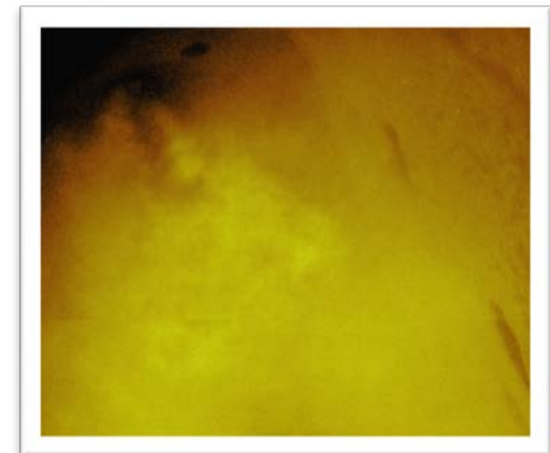
Flame image from combustion of PRB coal with CO 2 -enriched (18% O 2 )
